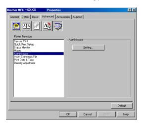
The Administrator selection permits the Copy, Scaling and Watermark features to be locked and password protected.
